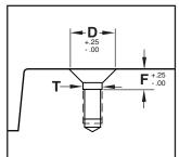
Microdaters can be installed directly into the plates or inserts or into a core pin or ejector pin with the material hardness around 35-40 HRC to utilize conventional machining methods.
