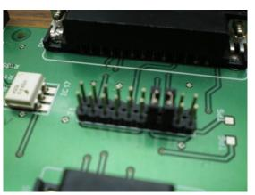
Protocol 20mA (-+) PASIVE (THE IMM "MASTER" PROVIDES THE POWER SUPPLY)
