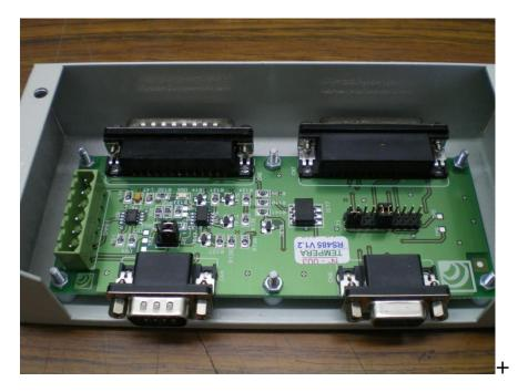
Configure the jumpers on the card of communications depend on the type of protocol that we will use.
