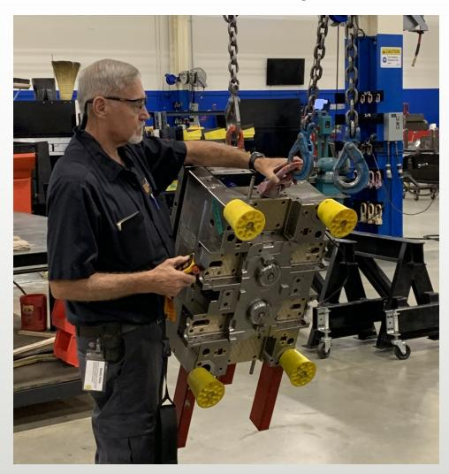
Rhino Feet are magnetic which means they can travel with the workpiece. Stick them on and leave them in place. Eliminate wood pallets and blocks from your shop!
